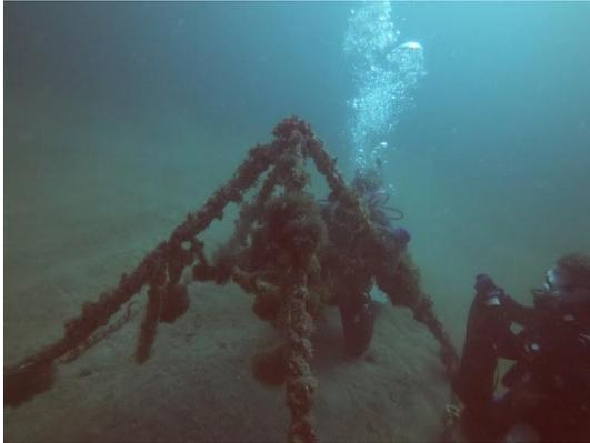
ARMS unit using current mounting system with 9 months growth at 20-meters depth
