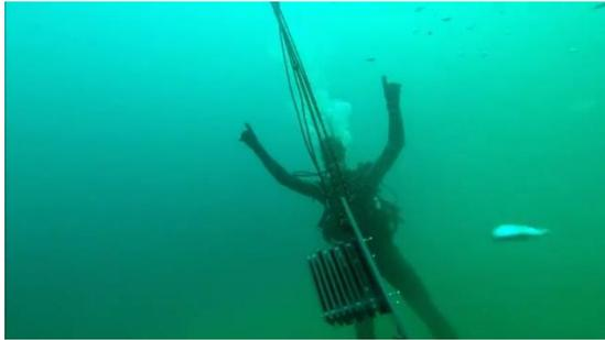
ARMS unit in final stage of original mounting system suspended in water column by 5 gal bucket filled with air
